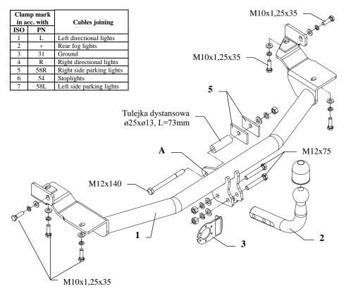
This towbar is designed to assembly in following car: **MITSUBISHI SPACEWAGON, VAN (N5, N8, N9),** produced since 11.1998 till 04.2004, catalogue no. **Z27** and is prepared to tow trailers max total weight **1600 kg** and max vertical load **80 kg**.
